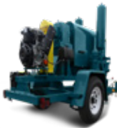
SLUDGE PRO® MOBILE DOUBLE DISC PUMPS Engine Driven Portable Sewage Pumps Size: 3", 4", 6" (76mm, 102mm, 150mm) Max Capacity: 371 GPM (23 lps) Max Head: 115' (35 m) Options: Tier 4 final diesel engines, trailer and skid packages
