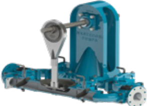
SLUDGE PRO® MOBILE DOUBLE DISC PUMPS Engine Driven Portable Sewage Pumps Size: 3", 4", 6" (76mm, 102mm, 150mm) Max Capacity: 371 GPM (23 lps) Max Head: 115' (35 m) Options: Tier 4 final diesel engines, trailer and skid packages
